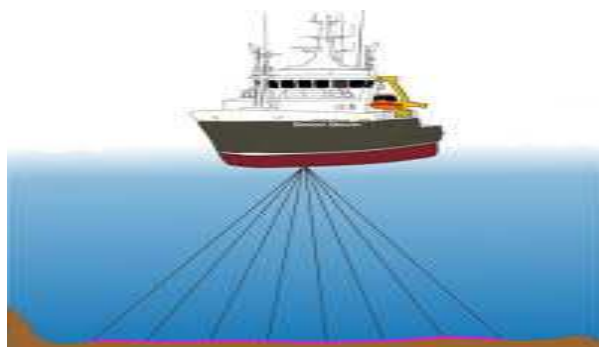
(Figure by VLIZ : Working principle of the multibeam)
